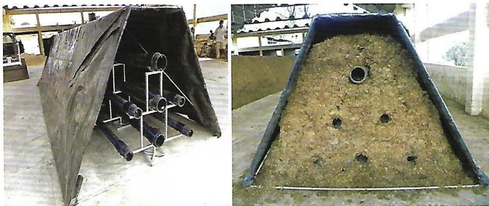
ZEPT method of composting with HDPE pipes in the compost pile
